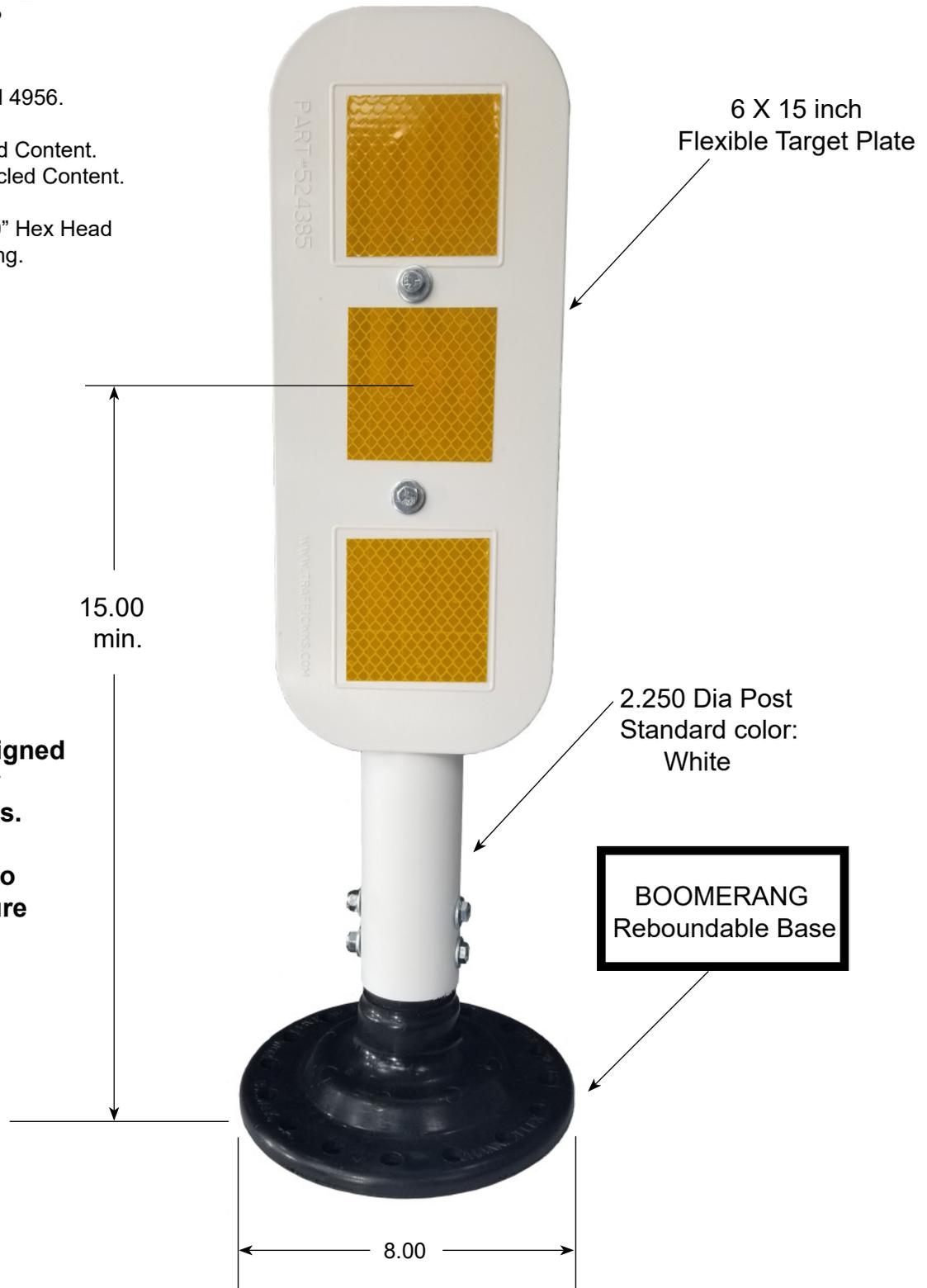
**Boomerang Base is designed to be impacted from any direction. All 360 degrees.**
